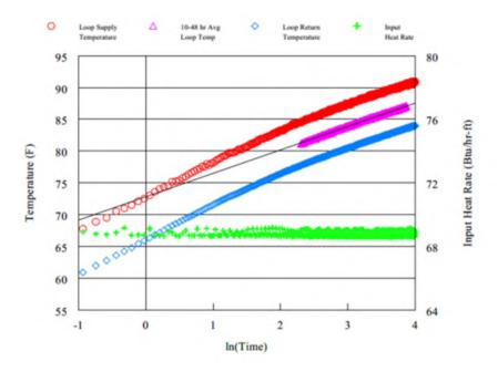
Figure 17: Thermal Conductivity Test Results
