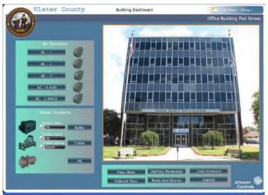
Figure 4: Johnson Controls Metasys Building Automation System
