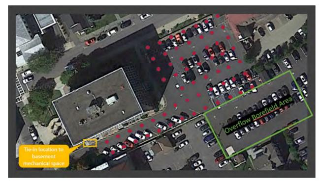
Figure 18: Heat Exchanger grid layout
